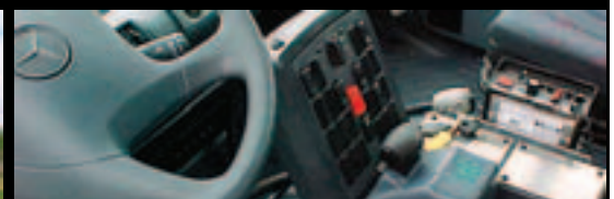
In cab pump panels
