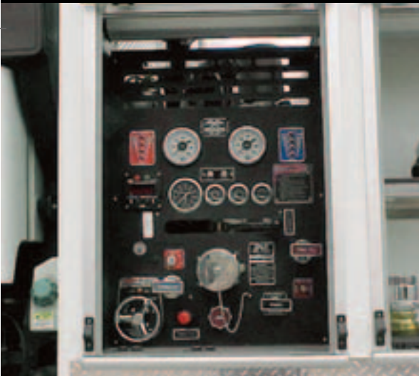
500 GPM pump with pump and roll
