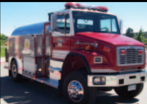
Tank capacities ranging from up to 2000 gal on a single rear axle to 3500 gal on a tandem.
