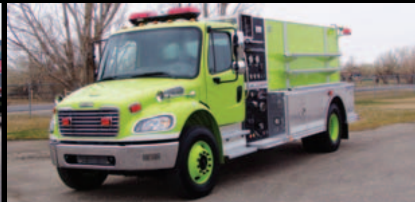
Freightliner M2 Chassis available to 66,000 lbs GVWR with power options up to 410 HP and seating for up to six
