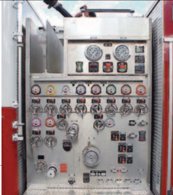
Brushed stainless steel pump module resists "rust" or "white" corrosion
