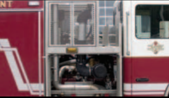
Swing away doors permit easy servicing of fluids and power plant - no need to tilt the cab
