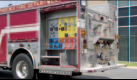
Simplified pump operations with color organized panels
