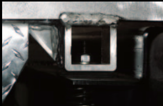
Spring loaded 4-point body mounting design reduces road shock transfer
