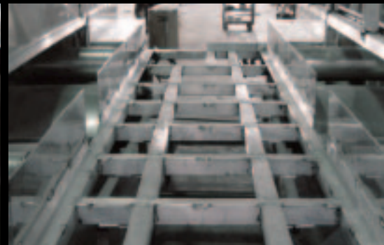
Body frame with integral tank support provides lasting strength
