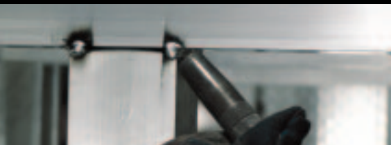
Extrusion framework design welds joints inside and out
