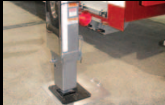
Out-and-down outriggers for tighter spaces
