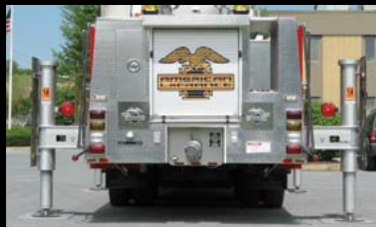
12" "H Style" Outriggers allow aerial operation at full capacity in tight areas
