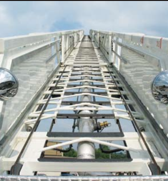
Clear unobstructed walkway with wider and deeper fly section
