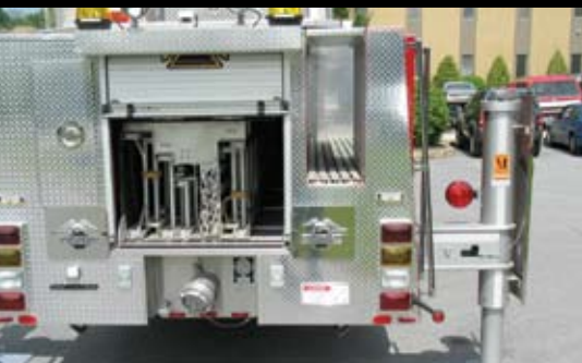
Low ground ladder storage with safe and easy access to hose and equipment
