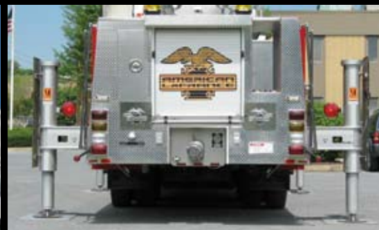
14" "H Style" Outriggers allow aerial operation at full capacity in tight areas
